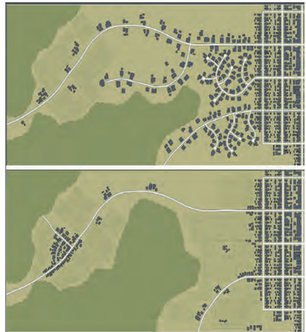
Clustering vs. diffuse home spacing in the WUI, Fire Mitigation in the Wildland Urban Interface. (source: 6 https://transect.org/modules.html ; accessed 10/30/23)
